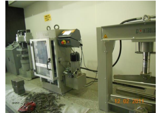
Compression, Split tensile, Flexure and bending testing
